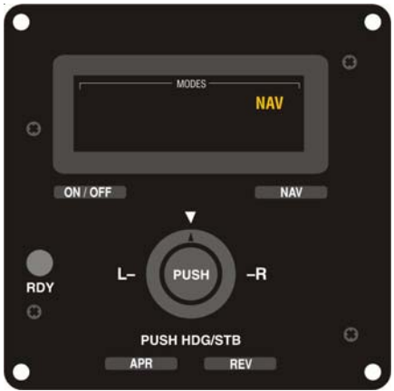
Fig. 2-7. AP Display, NAV Mode Engaged (System Forty)
