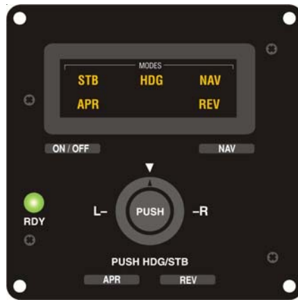
Fig. 2-1. AP Display, STB, HDG, NAV, APR, REV Annunciators Appear, RDY Lamp Illuminated (System Forty)
