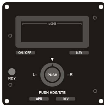
Fig. 2-2. AP Display, All Annunciators and RDY Lamp Extinguished (System Forty)
