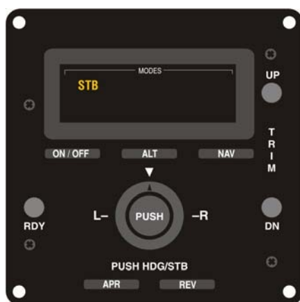
Fig. 2-17. AP Display, STB Mode Engaged (System Fifty)
