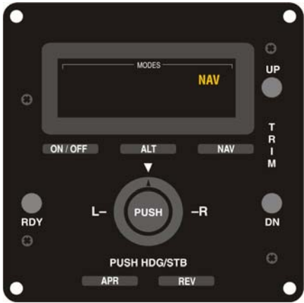
Fig. 2-19. AP Display, NAV Mode Engaged (System Fifty)
