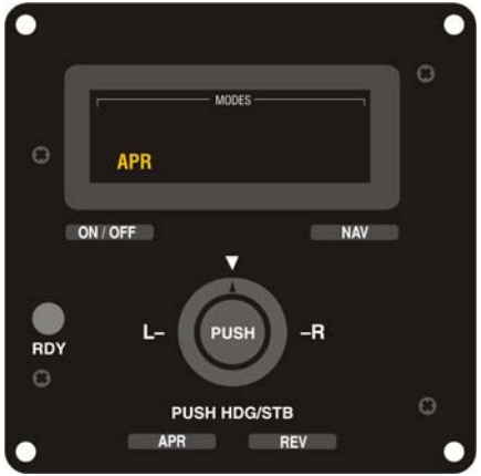
Fig. 2-8. AP Display, APR Mode Engaged (System Forty)
